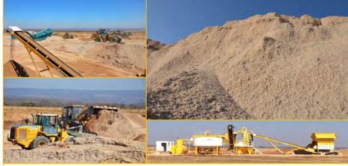
AST's pilot plant at Van Dykspruit is the first complete plant of its kind in South Africa. The modular design of the EvoWash system ensures highly accurate separation of organics, silts and clays from typical "Run of Mine" material. The plant ensures AST consistently produces exceptionally high-quality sand products.
